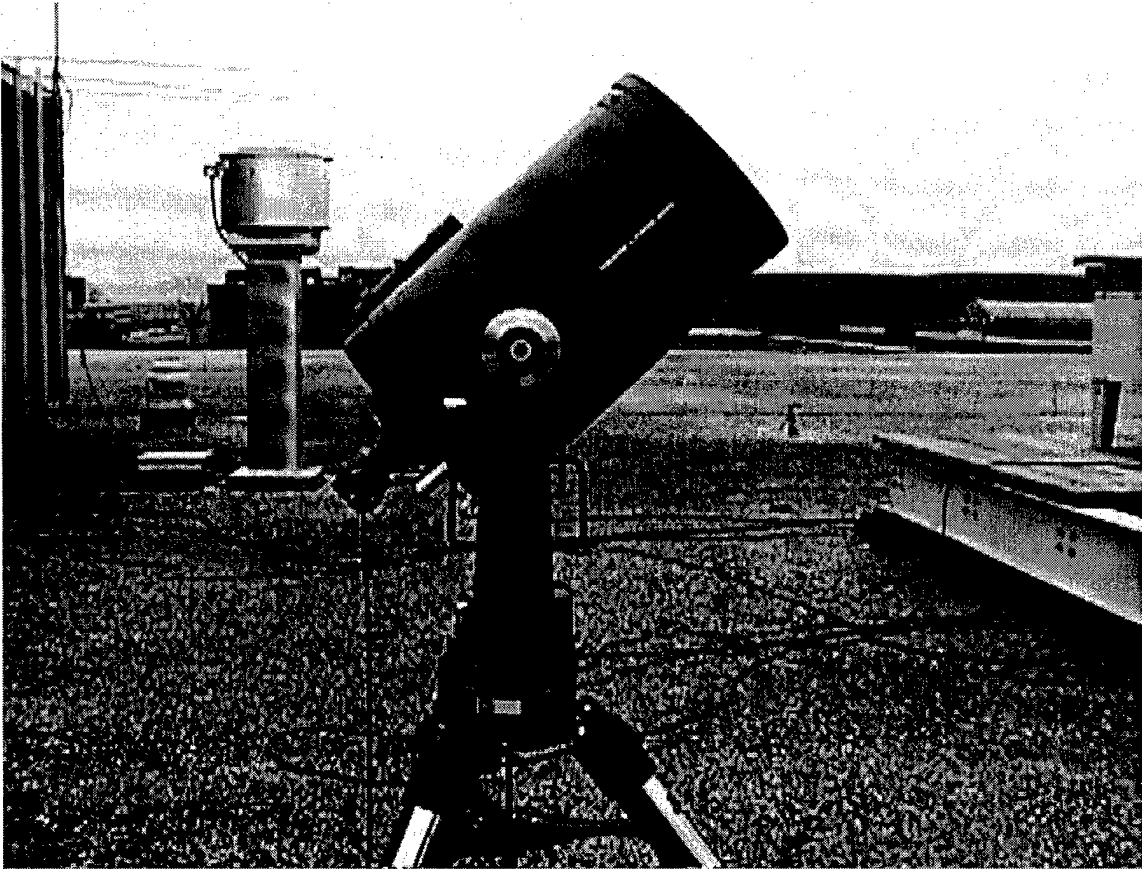
Figure 21. Picture of the Meade 12" diameter LX-200 Schmidt-Cassegrain telescope (with tripod). All attempts at capturing nightglow radiation were made with the telescope pointing to the zenith. The optic fiber is hanging from the smaller end.
